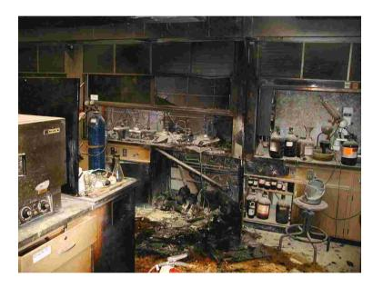
Explosion and Fire at Texas Tech University in 2001. A 4-L bottle of ether broke inside a fume hood and spilled onto a hot plate. The researcher was unable to extinguish the fire with two fire extinguishers and quickly exited safely.
